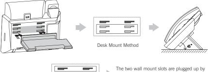
silica gels. You can pull out the silica gels when mounting your IP phone to a wall.
