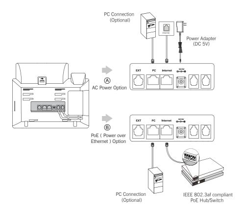
Note: If inline power (PoE) is provided, you don't need to connect the power adaper. Make sure the hub/switch is PoE-compliant.
