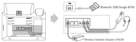
Note: The headset, Bluetooth USB dongle BT40 and wireless headset adapter EHS36 should be purchased separately. The EXT port can also be used to connect the expansion module EXP40. For more information on how to use the EHS36, EXP40 and BT40, refer to Yealink EHS36 User Guide, Yealink EXP40 User Guide and Yealink Bluetooth USB Dongle BT40 User Guide.
